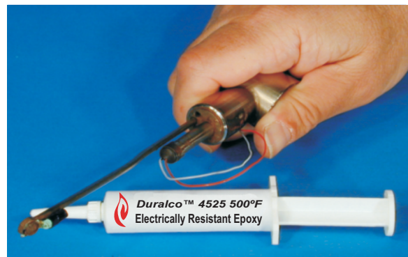
4525 Forms a Moisture Proof End Seal on an Electronic Sensor
