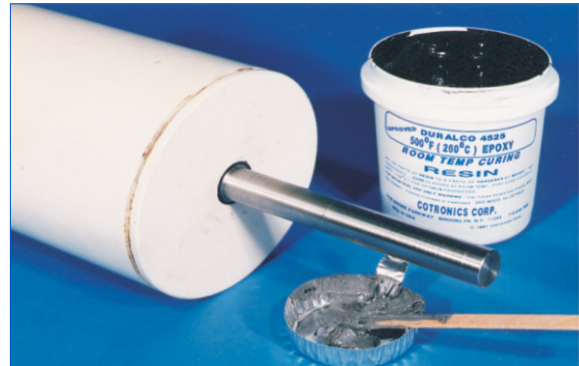
4525 Bonds a 316 S.S. Shaft to Repair the Ceramic Piston in a Hi-Temperature Acid Pump
