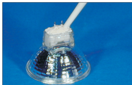
Production Potting of High Performance Light Bulbs
