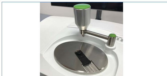
Figure 7: The Specac Arrow™ Silicon ATR crystal mounted in a Spectrum Two UATR.
